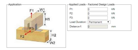
**Application** - This generic image is used to define the dimensions and load directions. This image is specific to each application type
