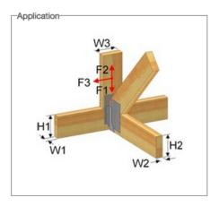
**Application** - This generic image is used to define the dimensions and load directions, which will change depending on the type of product and timber members that have been selected
